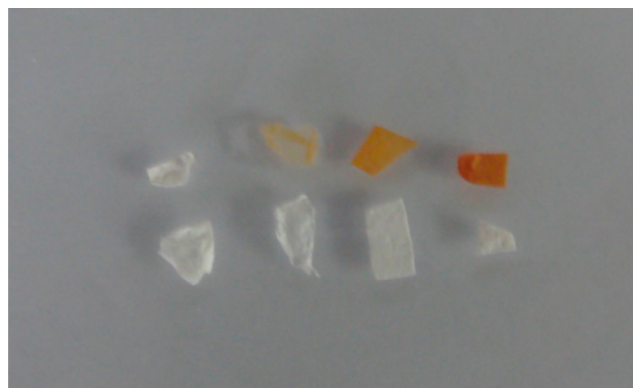
Figure 5. Image (from left to right) of PCL 80 , f-PCL-N 3 -20, f-PCL-N 3 -40, and f-PCL-N 3 -60 fibers after incubation with FITC-alkyne, with (top line) and without catalysts (bottom line), demonstrates successful attachment of the FITC fluorophore by click chemistry and macroscopically visible differences in the grafting ratio.
